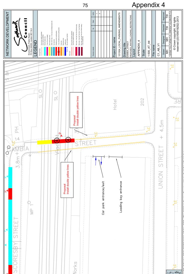
S:\NET\_DEV\01\_PROJECTS\2006\_07\C1\_CPZ\_4TH\_2006\11 Design Drawings\04 As Built\C1\_AB\_V1.2.dwg
